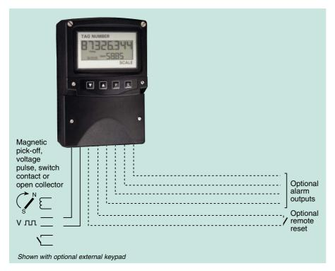
The BA544D is a battery powered rate totaliser with separate rate and total displays. An accumulated grand total may also be displayed. The instrument will count switch contact closures, voltage pulses and the low level output from magnetic pick-offs.
